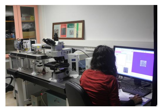
The system is capable of capturing high speed (30fps, 512x512) or time-lapse (seconds to hours) confocal data sets from low light emitting specimens. There is also an in-line specialized FRAPPA unit for monitoring fast (msec) multi-point FRAP/FRET events. It does this by combining Yokogawa CSU-XI spinning disk head and an Ixon+ back-illuminated EMCCD camera (Andor) coupled to an Olympus BX61 upright microscope. Location: room 112 Fruit Three building Plant Science institute.
